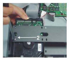
Second, attach the HDD by two screws on both
